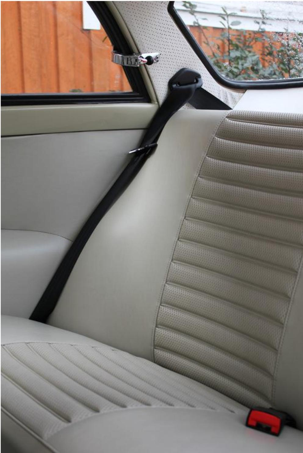
Two holes in the roof vinyl, slits in the rear shelf mat/paper and holes drilled in the wheel housing are the permanent changes made to the car using this solution. The result is good and above all safe.
